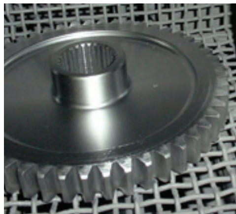
Fig. 1. Vacuum carburized 8620 gear
